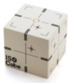
ISO Cube is a routine phantom made from water equivalent material for testing of positioning, alignment and isocentre checks of CBCT imaging systems, in both kV (imaging) and MV (treatment) energy ranges. This phantom is supplied with an alignment plate for fast & easy set up.
