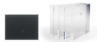
PIXMAM is a digital mammography image quality phantom comprising a stack of finely toleranced PMMA plates.
