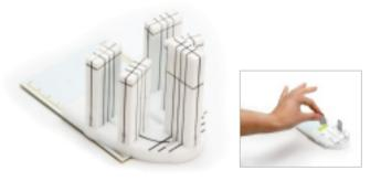
A test object that allows the complex focal trough of the panoramic x-ray unit to be quantified, as well as the capacity for spatial resolution testing using line-pair test patterns (available separately) and contrast resolution insert (available separately).
