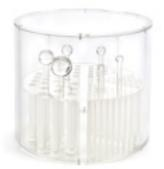
SPECT IQ is designed for checking image quality performance of SPECT systems.
