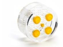
MagIQ 142 is an image quality phantom for Magnetic Resonance Imaging (MRI) comprising a main chamber and four 'test tubes' which may be filled with different solutions to create a total of 5 separate signal compartments.
