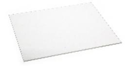
Rigid PMMA phantom for the quality control of geometric distortion and spatial resolution of gamma cameras.
