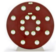
Tissue Equivalent phantom consisting of a water equivalent nested head and body phantom each with 8 holes to house interchangeable inserts of different tissue equivalent materials as follows:
