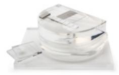
TO PASMAM is designed to be used to check the image quality performance of digital mammography systems, both on commissioning and on a routine basis.
