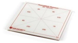
A routine test object designed to provide an ongoing check of the resolution of fluoroscopy systems. Image quality is measured simply by counting the number of mesh patterns resolved in the image.
