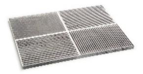
Rigid PMMA and Pb bar phantom for the quality control of spatial resolution of gamma cameras. The Gamma resolution phantom consists of four sections, each with different bar dimensions, and features engraved, pigment filled centre lines for accurate and repeatable positioning.
