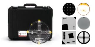
A QA test phantom for magnetic resonance imaging comprising a single chamber (MagIQ) or two identical chambers (MagIQ Duo), which may be filled with different solutions to create two test objects (e.g. high field and low field). Automated scoring software is available separately.
