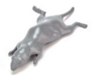
The Leeds MicroCT Mouse Phantom is a tissue mimicking, pontikiomorphic (in the form of a mouse) phantom for use in demonstrating and assessing image quality of pre-clinical MicroCT scanners.
