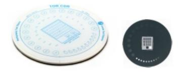
A routine QA test phantom for radiography systems.TOR CDR is used to provide an ongoing check of imaging performance, particularly those aspects which are most liable to deterioration. Used for conventional, computed and digital radiography.
