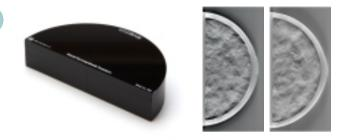
A breast tissue simulating test object designed to be used to compare image quality between different exposure parameters within a single system or across different breast tomosynthesis systems.
