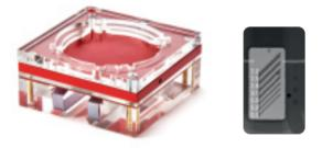
TOR DEN Digital is designed to be used to check the image quality performance of digital intra-oral x-ray systems.
