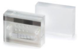
Leeds Test Objects' DENTEST phantom is designed to be used to check the image quality performance of digital intra-oral dental x-ray systems. These test should be carried out on commissioning, and on a routine basis to check for any deterioration in performance.
