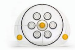
Leeds Test Objects' PET IQ Phantom is a realistic anthropomorphic PMMA vessel, which simulates the trunk of the human body.
