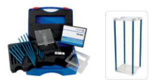
The TO HVL filter stand is designed for use with any X-ray system. This test object (when used with an appropriate set of Al filters and a multi-meter) allows the user to test the half value layer (HVL) of their x-ray system.
