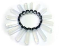
A set of 18 gel-filled tubes with calibrated T1 and T2 values, sized to insert into the contrast sections of MagIQ Solo and MagIQ Duo phantoms.
