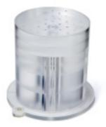
The SedentexCT Dose Index (DI) phantom comprises a stack of PMMA plates forming a cylinder representing the adult head. Several types of detector systems are catered for:
