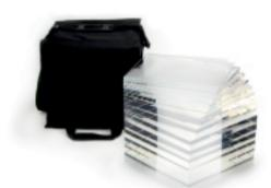
TO AEC is an x-ray quality assurance phantom comprising a stack of PMMA plates which allow the user to check the consistency, repeatability and reproducibility of AEC system function.
