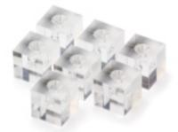
A set of 7 clear PMMA cubes, 17x17x17mm, with a 5mm dia. spherical fillable void, which can be filled with any mixture of radionuclide, CT contrast agent or MR contrast agent and sealed with a nylon screw (provided).
