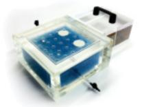
The Harefield VQ SPECT is designed for checking image quality of SPECT systems using perfusion ventilation (VQ) with isotopes Tc-99 and Kr-81.
