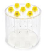
MagIQ Diffusion is used for calibration of contrast values when performing Diffusion Weighted Imaging (DWI) and Apparent Diffusion Coefficient (ADC) imaging protocols.
