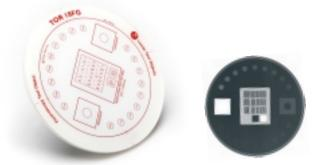
A routine QA test phantom for fluoroscopy systems. TOR18FG is used to provide an ongoing check of imaging performance, particularly those aspects which are most liable to deterioration.
